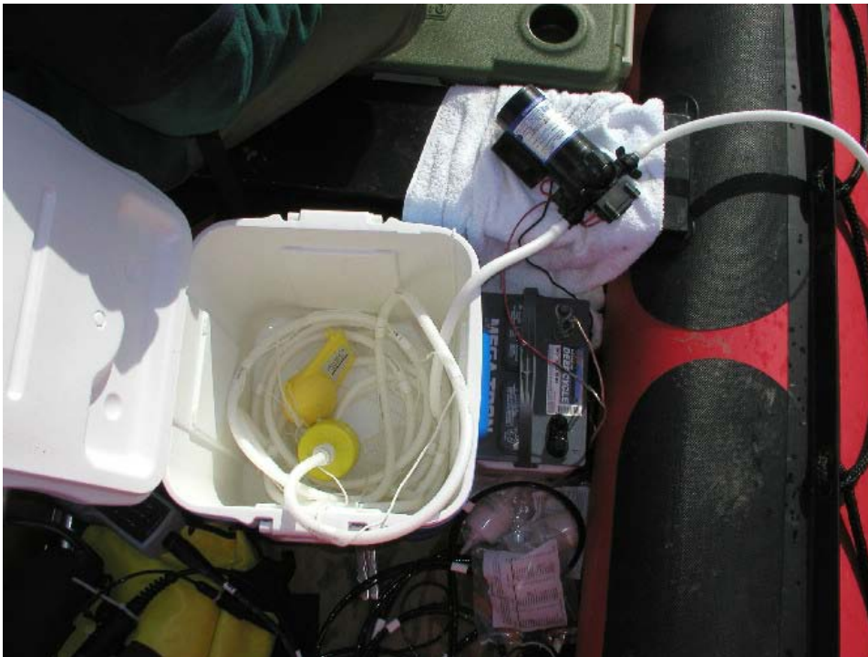
Photograph 1: Use of clean cooler to protect sample inlet line and hydro weight from contamination when sampling from a boat. Round yellow object on end of C-flex tubing is plastic screen to prevent end of inlet line from touching sediment or sucking in debris.
