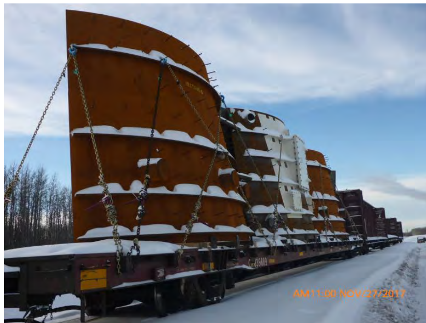
Figure A-8 Draft Tube Elbow Sections Delivered via Rail Car. Photo taken November 27, 2017.
