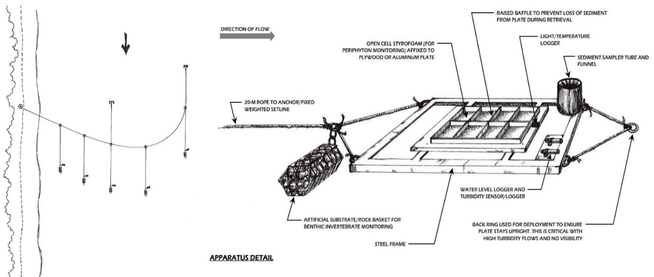
**Figure 2-2: The typical deployment (left) of the sampling apparatus (right) used.**
