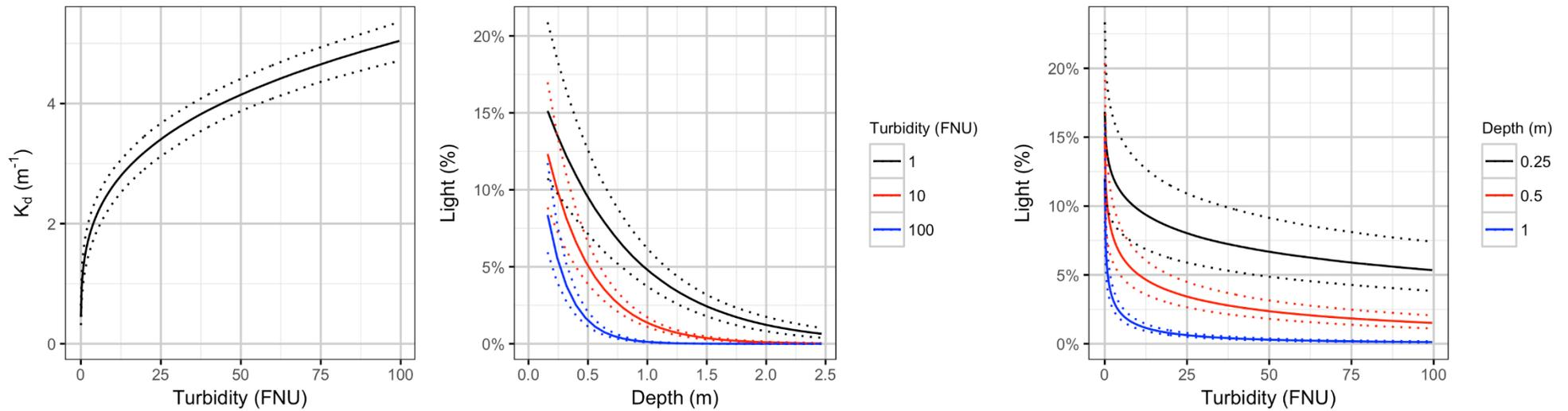
**Figure 3-1:** The left figure shows the relationship between the diffuse light attenuation coefficient and the turbidity. The middle figure shows the relationship between the light attenuation and the depth at 1 FNU. The right figure identifies the relationship between the light attenuation at 0.2 m and the turbidity. Dotted lines represented 95% Confidence Limits (CLs).
