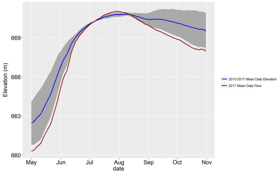
**Figure A14** Water Elevations in Williston Reservoir at Williston Forebay 1.
