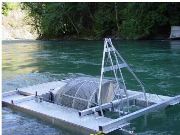
*Photo of a rotary screw trap in operation*
