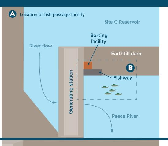
Migratory fish are naturally attracted to fast-flowing water, and with this in mind, BC Hydro located the permanent fish passage facility at the outlet of the generating station, where fish will be attracted to the high flows exiting the turbines.
