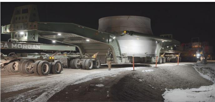
A convoy carrying a 170-tonne turbine runner on its way to the Site C project. A turbine runner is the portion of the turbine that is in contact with the water and acts as a water wheel to turn the generator. Six runners will be used in the hydroelectric project. See more project photos in the <u>image gallery</u>.
