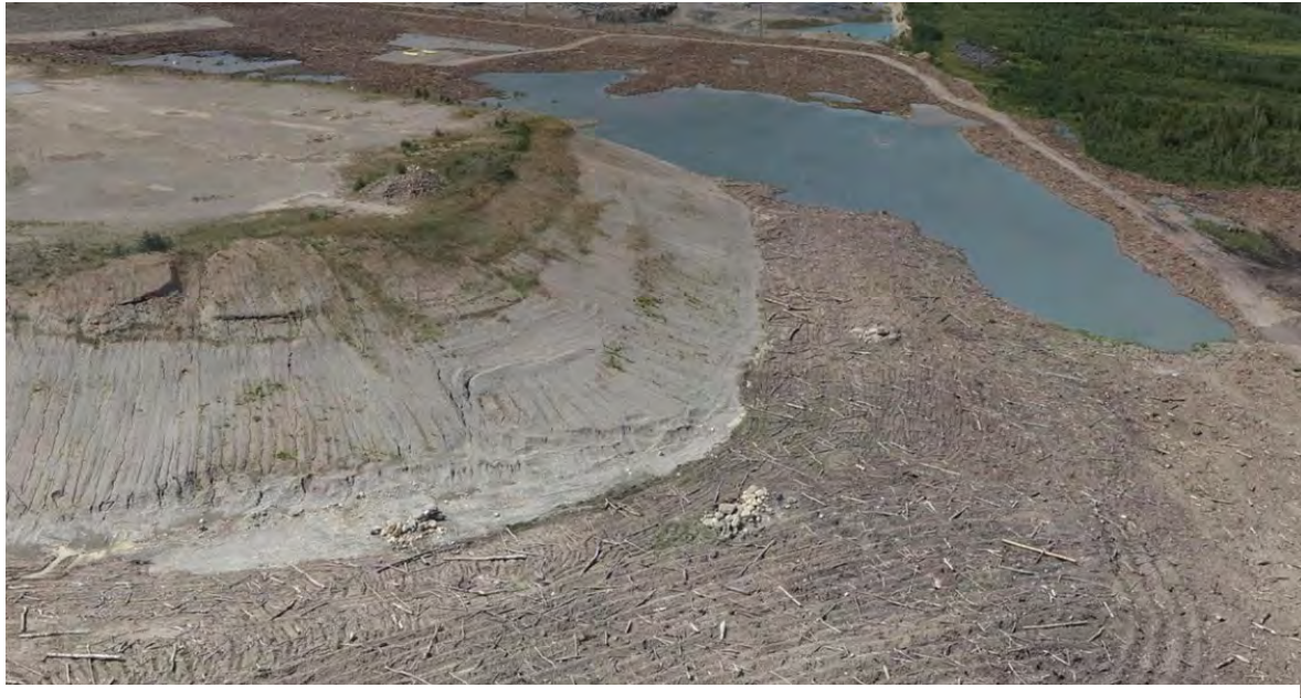
Figure 17. Aerial drone photo of Basin 3 showing the wetland created in this section with distribution of coarse woody debris. This area has also been seeded so vegetation will be expected to grow in over time. Photo taken in August 2024.
