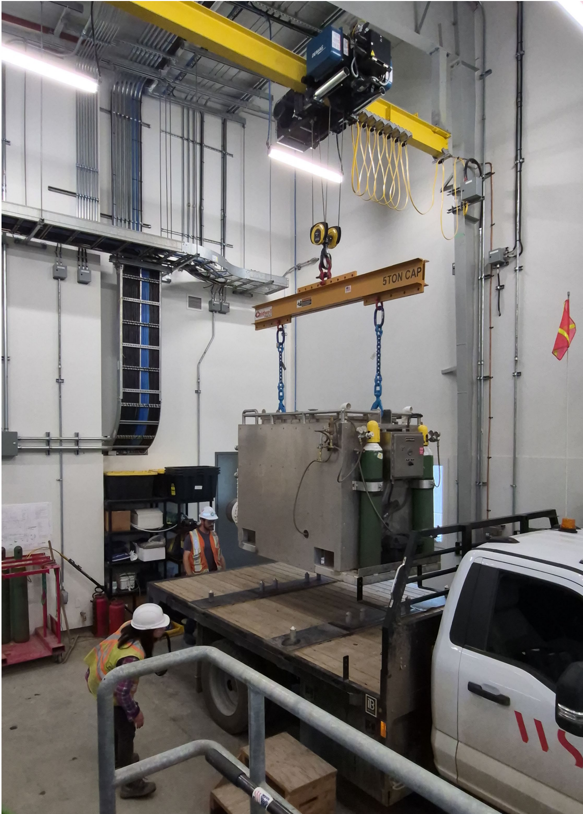
Photo 3. Operator uses the monorail crane hoist to lower a transport pod full of water and fish onto the back of the transport truck (August 5, 2025).
