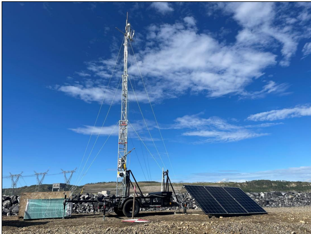
Figure 3.2 Dam EC System photograph
