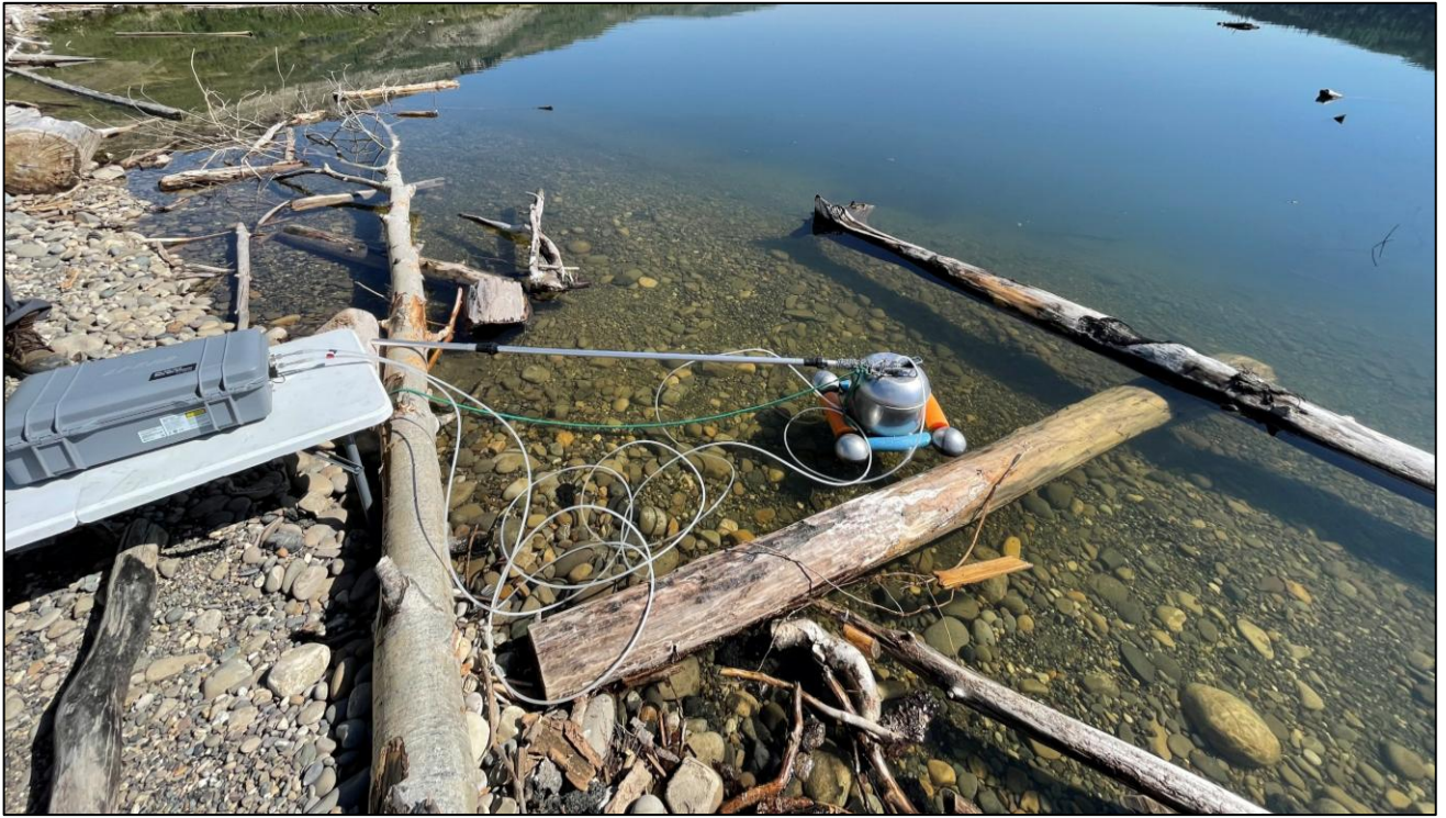
Figure 3.7 Photograph of flux chamber and gas analyzing during sampling
