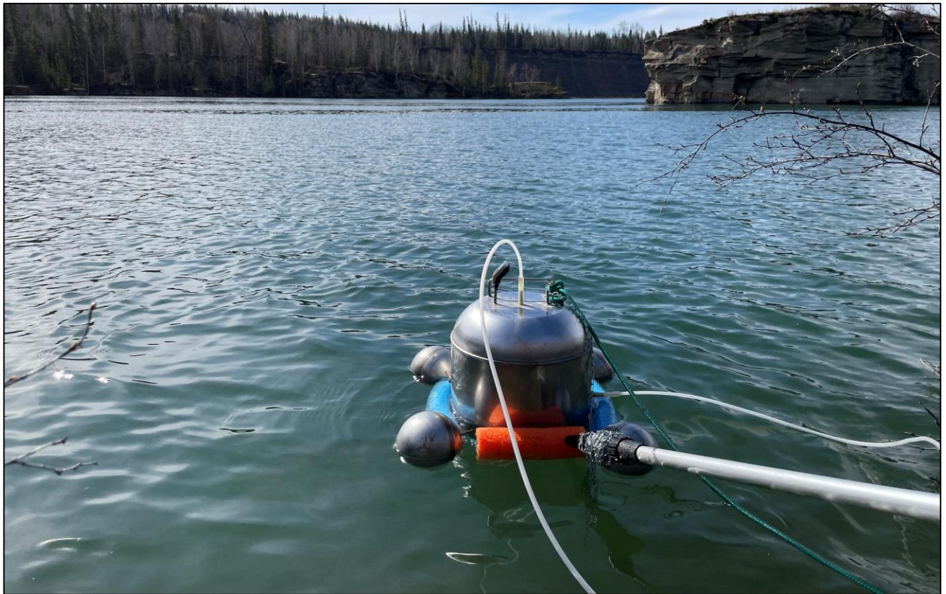
Figure 3.8 Photograph of flux chamber during sampling
