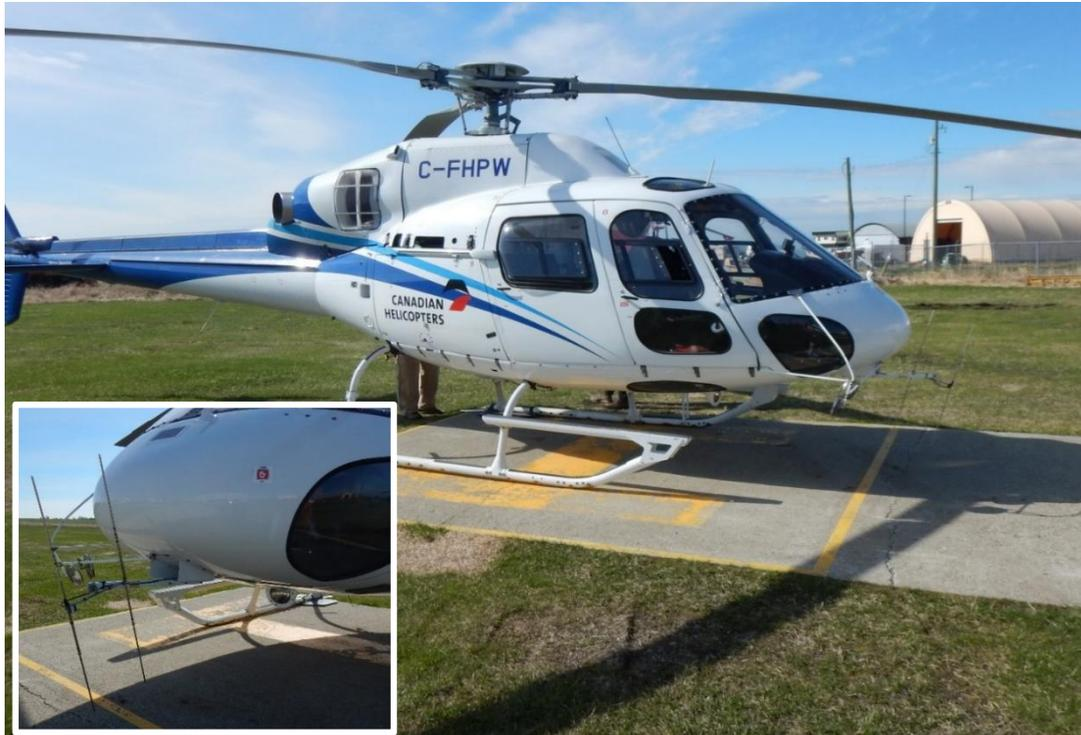
Figure 3. Twin-engine helicopter equipped with a single H-antenna mounted on the nose for conducting mobile-tracking surveys in the Beatton River, 2021-2022.
