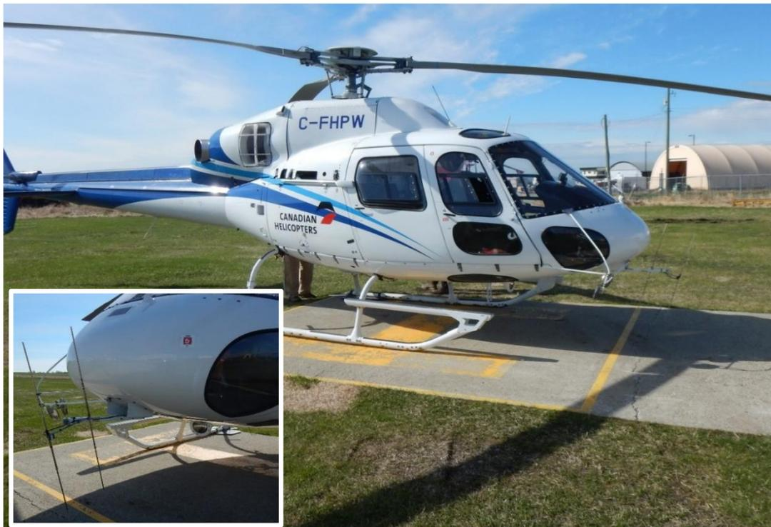
Figure 5. Twin-engine helicopter equipped with a single H-antenna mounted on the nose for conducting mobile-tracking surveys in the Beatton and Kiskatinaw rivers, 2021.
