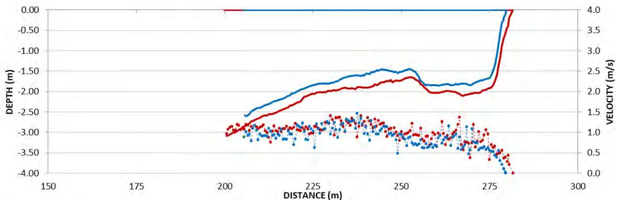
**Figure 9.** Water depth (solid lines) and velocity profiles (dashed lines) from August (blue) and October (red) measurement for transect profile GMS02.
