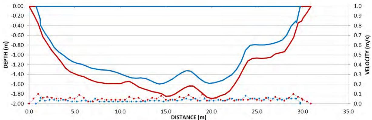
**Figure 4.** Water depth (solid lines) and velocity profiles (dashed lines) from August (blue) and October (red) measurement for transect profile GME01.
