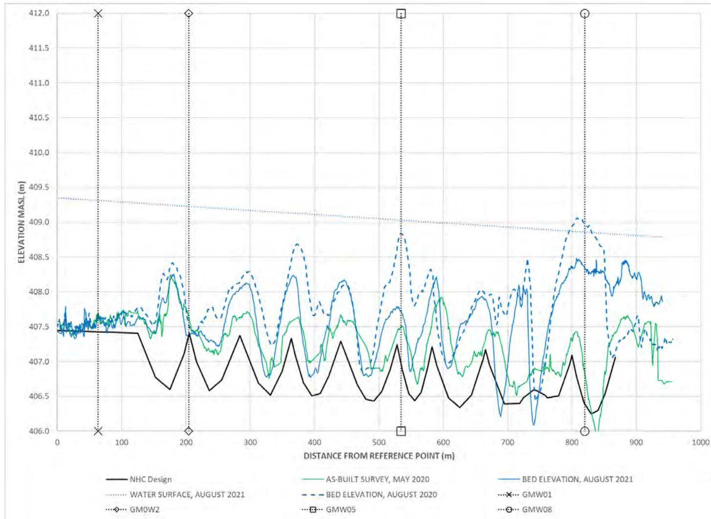
Figure 9. Plots of Main Channel Bar longitudinal bed profiles and water surface elevations for 2020 (top) and 2021 (bottom) surveys. Also shown are the Main Channel Bar bed profile in the as-built survey (May 2020) and NHC bed design, and location of transects.
