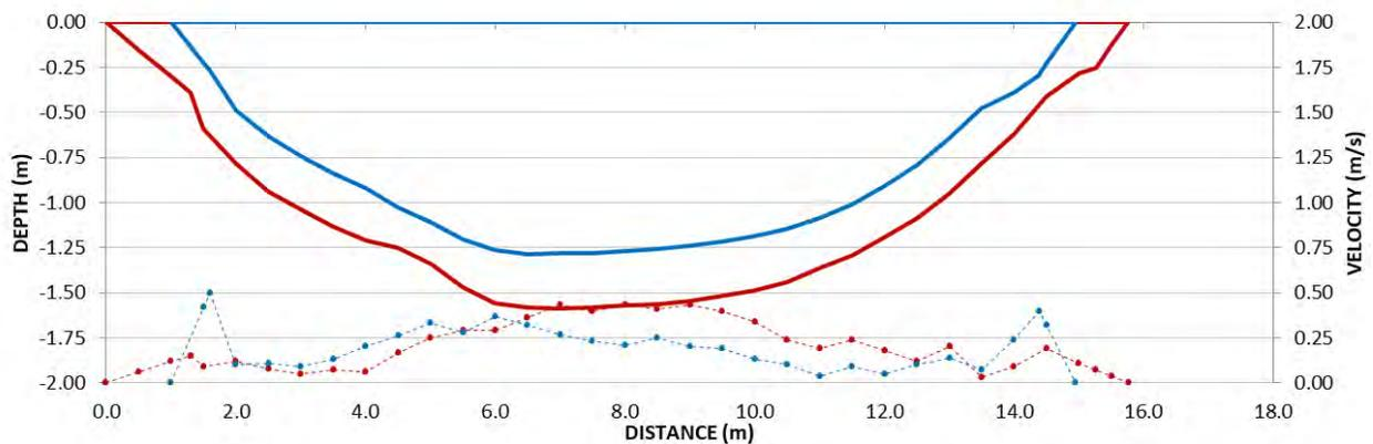
**Figure 6.** Water depth (solid lines) and velocity profiles (dashed lines) from August (blue) and October (red) measurement for transect profile GME03.
