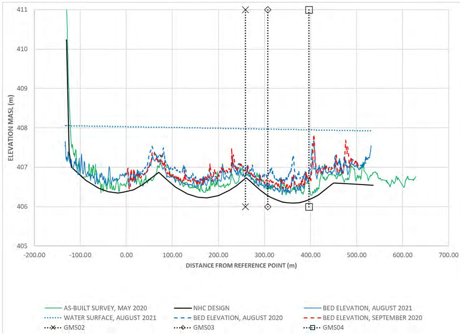
Figure 7. Plots of East Side Channel longitudinal bed profiles and water surface elevations for 2020 (top) and 2021 (bottom) surveys. Also shown are the East Side Channel bed profile in the as-built survey (May 2020) and NHC bed design, and location of transects.
