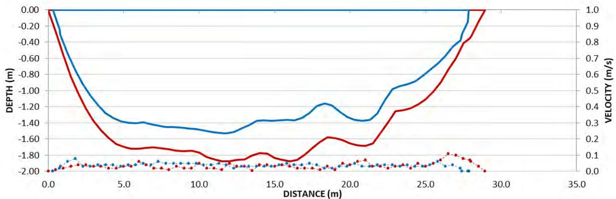
**Figure 3.** Water depth (solid lines) and velocity profiles (dashed lines) from August (blue) and October (red) measurement for transect profile GMB05.
