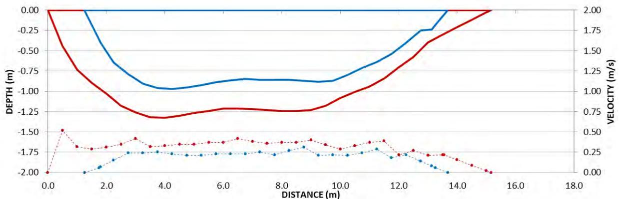
**Figure 7.** Water depth (solid lines) and velocity profiles (dashed lines) from August (blue) and October (red) measurement for transect profile GMP02.
