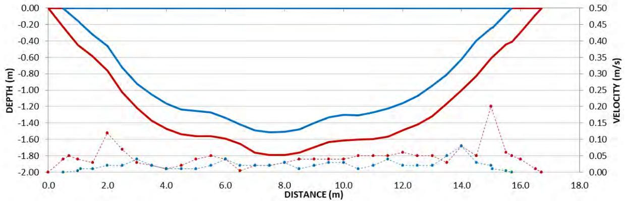
**Figure 11.** Water depth (solid lines) and velocity profiles (dashed lines) from August (blue) and October (red) measurement for transect profile GMS04.
