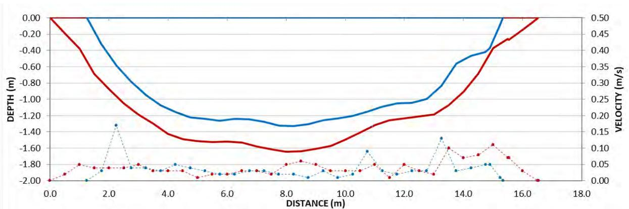
**Figure 12.** Water depth (solid lines) and velocity profiles (dashed lines) from August (blue) and October (red) measurement for transect profile GMW01.
