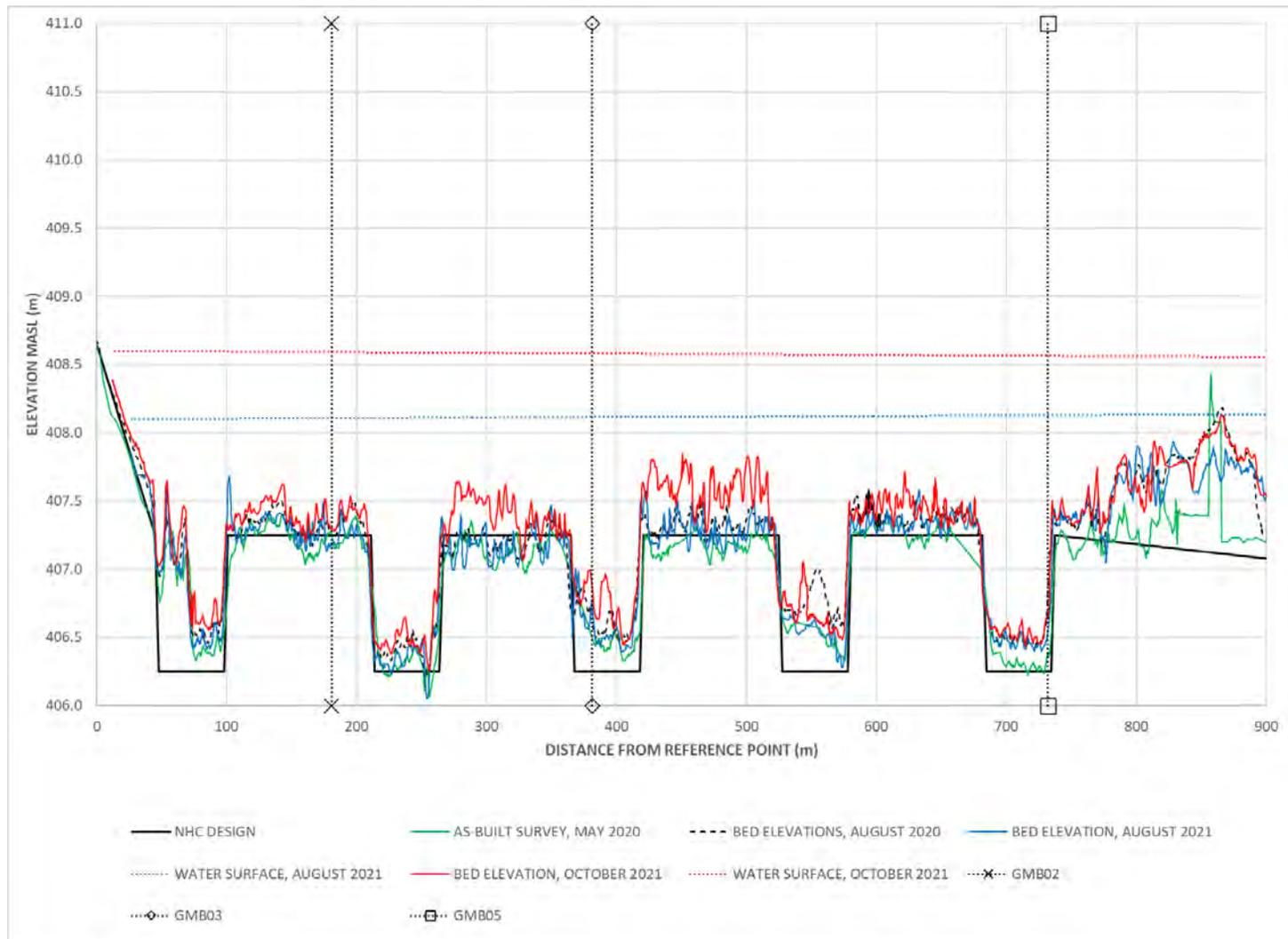
Figure 6. Plots of South Side Channel Spur Extension longitudinal bed profiles and water surface elevations for 2020 (top) and 2021 (bottom) surveys. Also shown are the South Side Channel Spur Extension bed profile in the as-built survey (May 2020) and NHC bed design, and location of transects.
