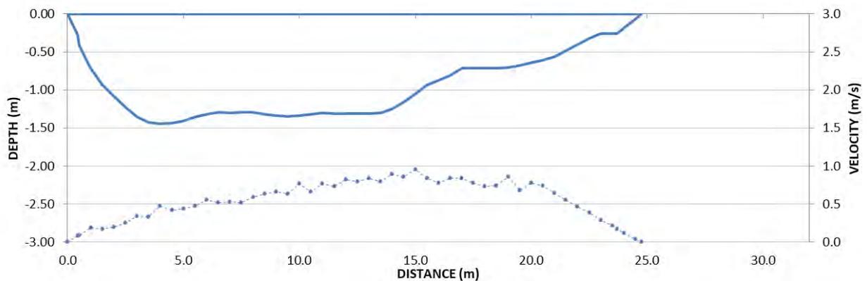
**Figure 15.** Water depth (solid lines) and velocity profiles (dashed lines) from August (blue) and October (red) measurement for transect profile GMW08.
