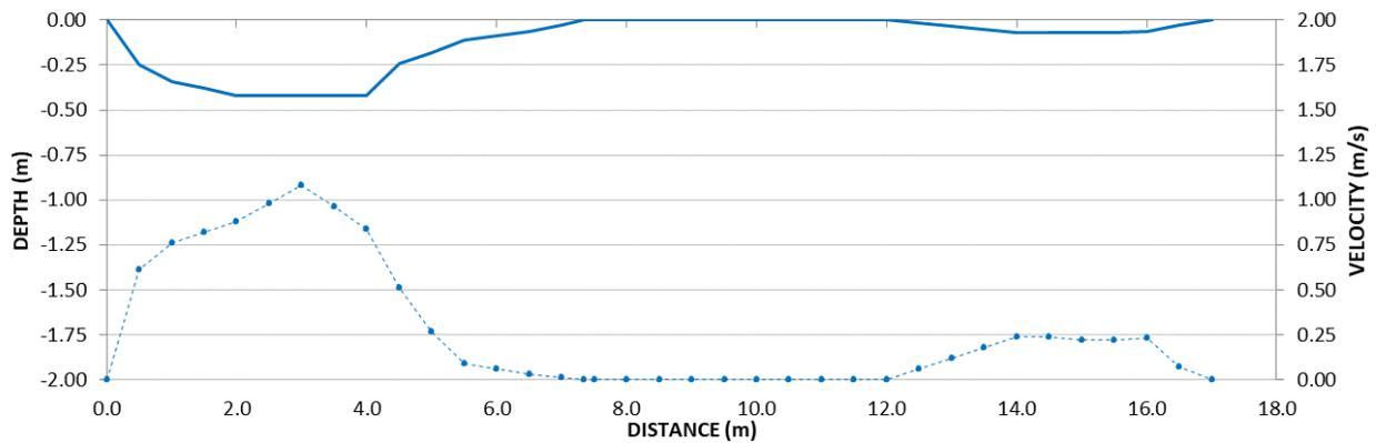
**Figure 5.** Water depth (solid lines) and velocity profiles (dashed lines) from August (blue) and October (red) measurement for transect profile GME02.
