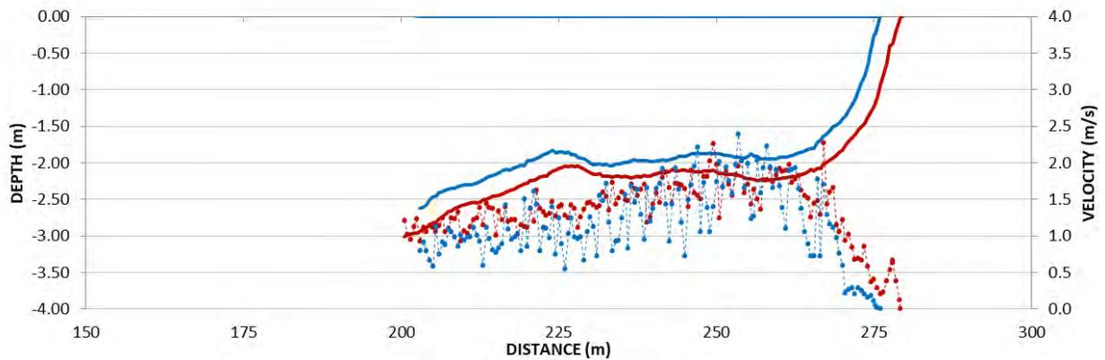
**Figure 8.** Water depth (solid lines) and velocity profiles (dashed lines) from August (blue) and October (red) measurement for transect profile GMP04.
