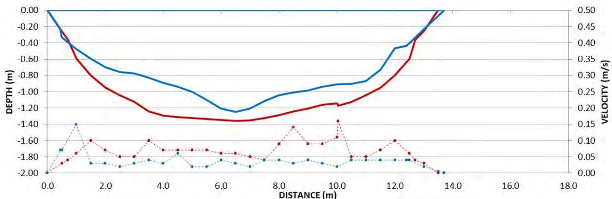
**Figure 10.** Water depth (solid lines) and velocity profiles (dashed lines) from August (blue) and October (red) measurement for transect profile GMS03.
