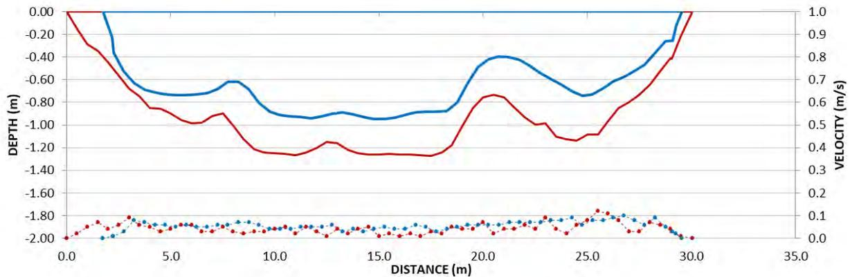
**Figure 2.** Water depth (solid lines) and velocity profiles (dashed lines) from August (blue) and October (red) measurement for transect profile GMB03.
