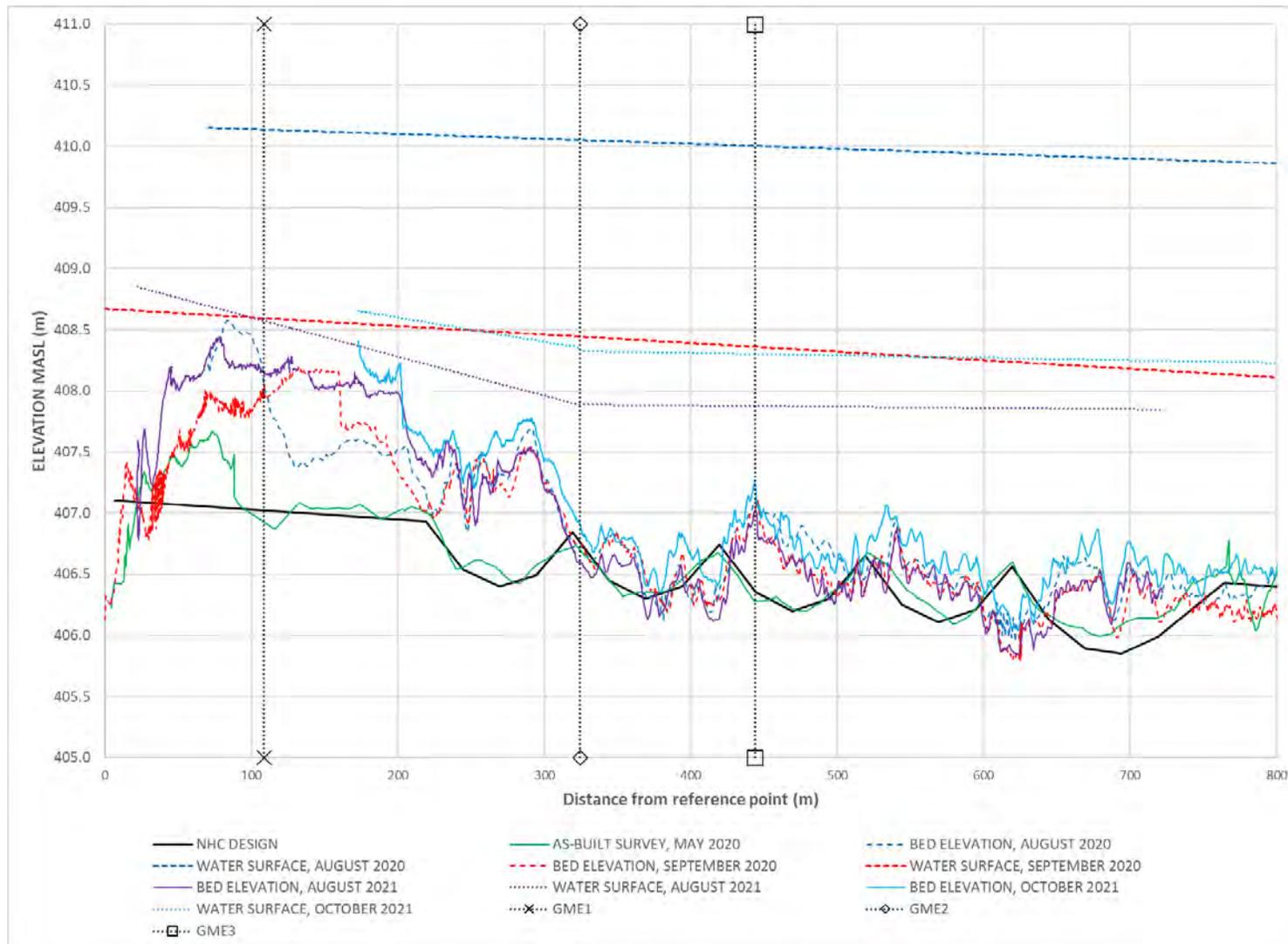
Figure 8. Plots of West Side Channel longitudinal bed profiles and water surface elevations for 2020 (top) and 2021 (bottom) surveys. Also shown are the West Side Channel bed profile in the as-built survey (May 2020) and NHC bed design, and location of transects.
