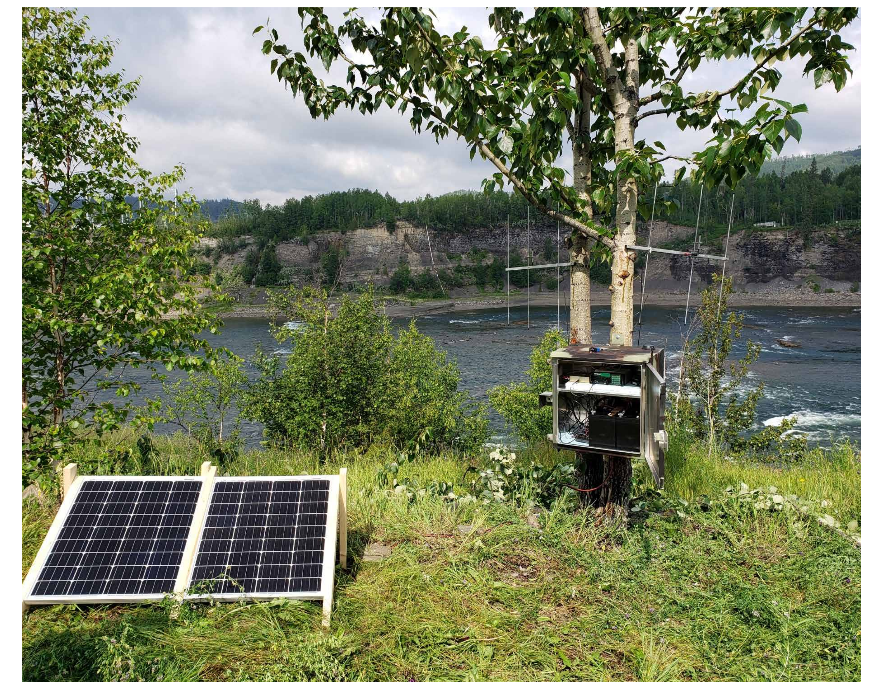
One of 30 new fixed telemetry stations placed on the river bank, which monitors the movement of radio-tagged fish.
