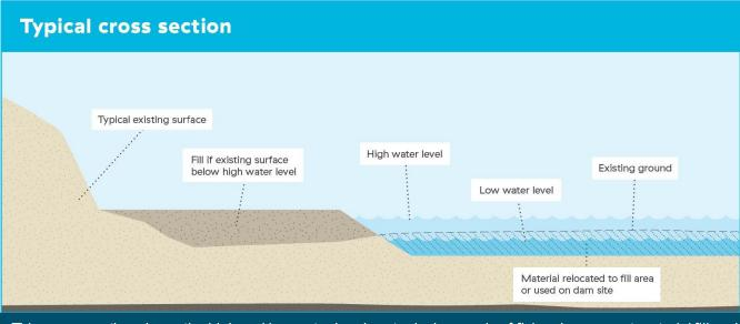
This cross section shows the high and low water levels, a typical scenario of fish enhancement material fill and removal.
