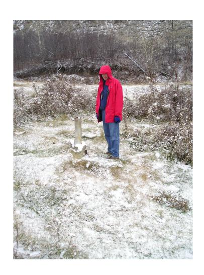
Site C3 – On the Left Bank where more drill hole casings have moved since they were installed due to ground movements.
