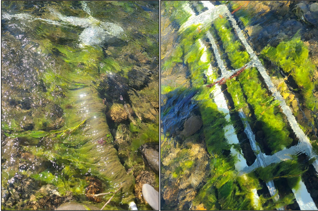
Algae or macrophytes (species unknown) entangled in Cypress Creek PIT antennas (left) and resistivity counter pads (right).
