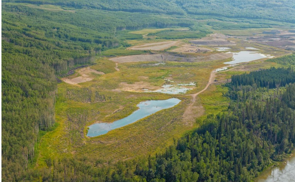
Figure A-17 Three wetland basins have been completed on the right bank, downstream of the dam. As planned, the wetlands are now gradually filling with ground water. (July 2025)
