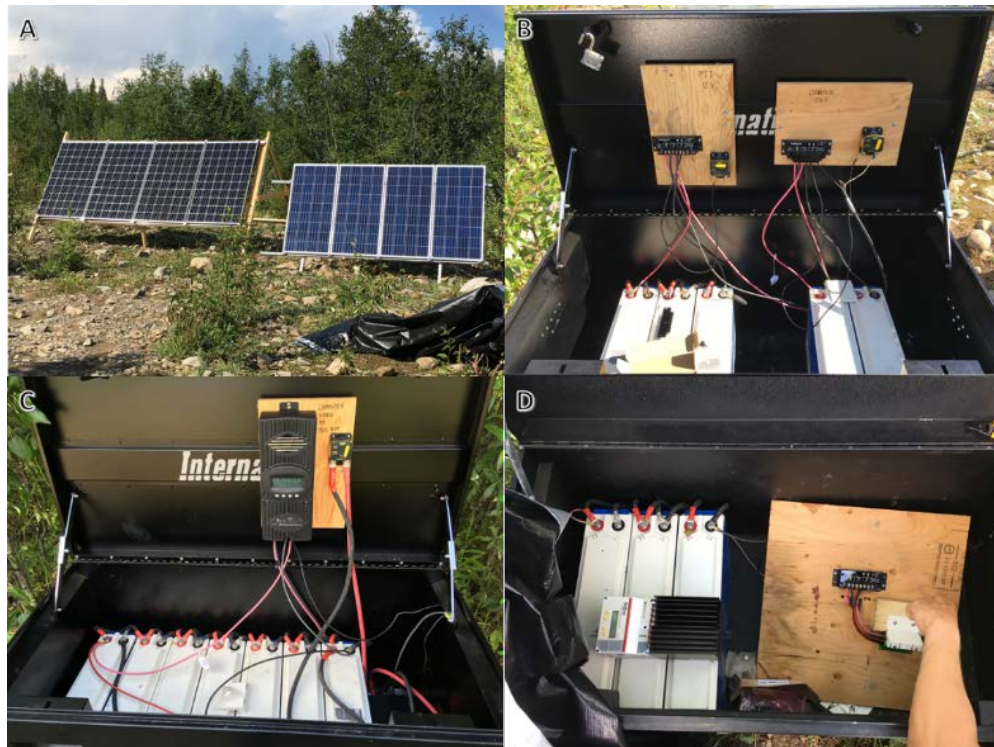
Figure 2-1. Power system configurations used in Cypress Creek, 2018. Panel A shows the solar panel setup, panel B depicts the upstream PIT reader and counter battery bank, panel C the video validation and computer battery bank, and panel D depicts the downstream PIT antenna battery bank. A similar configuration was used in the Chowade River.
