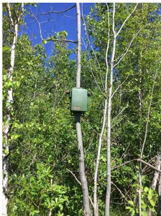
Photo 8 Example Deployment of an SM4 Autonomous Recording Unit with Internal Microphones for Bioacoustics Monitoring of Marsh Birds within Wetland Habitats
