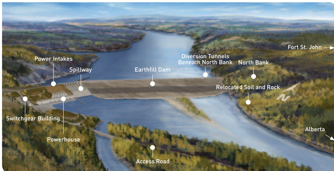
Major components of the Site C dam site (historic conceptual design).
