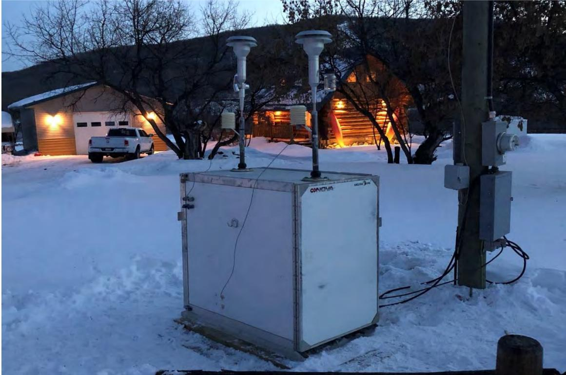
Figure 2-2: Upgraded Station 8 (Old Fort) with climate-controlled enclosure
